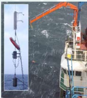
Figure 5. The tethered buoy. Main image: The buoy rides freely up and down a central, weighted, cable supported here by the aft crane, which keeps it in position. Inset: the buoy being lifted over the side of the ship – the CLASP inlets are visible above the flotation ring; the bubble imaging system is suspended beneath.
