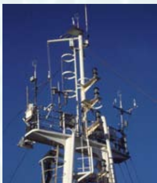
Figure 3. The flux instrumentation on the foremast of the Discovery : the NOC sonic anemometers are mounted at either side of the mast platform with LiCORs situated just below and forward. The Leeds sonic is mounted on the leading edge of the plate at the top of the mast with a LiCOR just aft. The CLASP units are mounted flat on the plate with inlets collocated with the licor.
